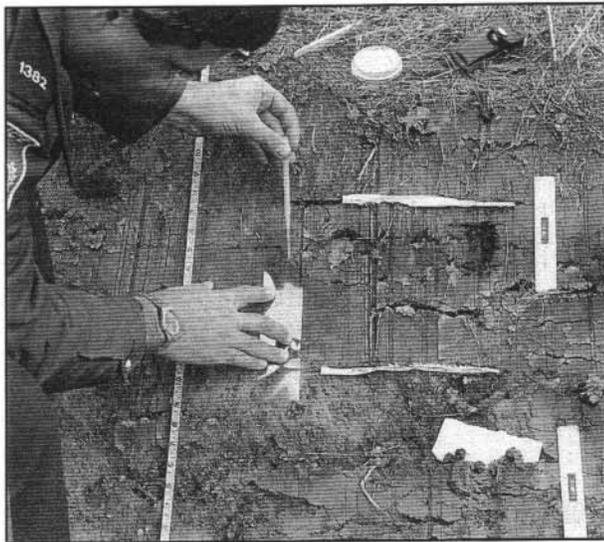
Samples can also be obtained by using an acetate sheet and acetone. Place a sheet over the area to be sampled and with a dropper, place acetone between the sheet and soil. Hold the sheet firmly at the base and continue to flood in an upward motion. Care should be used so as to not wash out the actual horizon with the acetone.
