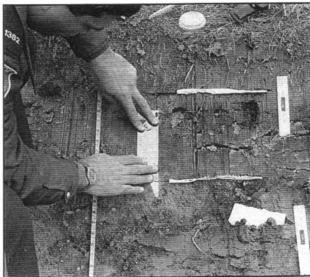
Once the soil face is suitably moistened with the acetone, hold the sheet firmly onto the face until the acetone evaporates. During this stage, the acetone is actually melting the acetone sheet enough to allow particles to be melted into and onto the sheet.
