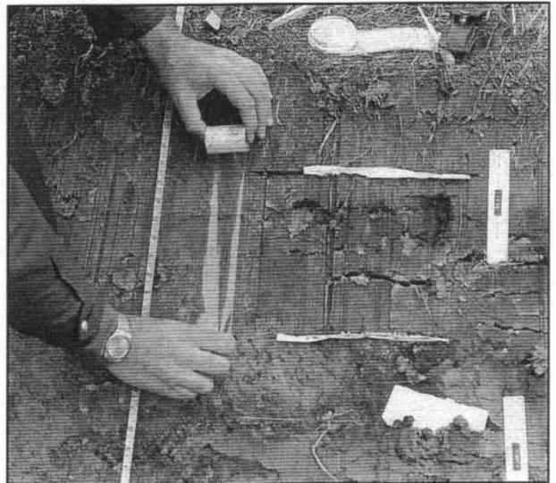
Once the tape is placed on the acetate sheet, the "lift" is then suitable for immediate microscopic examination. This method allows for any hair and fibre evidence that may be on the soil to be recovered as well. Some sandy soil types may impair the ability of the tape to adhere to the acetate. Should this occur, a cover strip of wider tape can then be placed over the sample to retain any loose grains.
