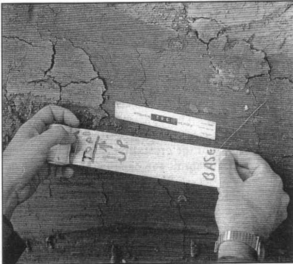
The labelling of the lift is of extreme importance. The lift should be marked in a manner to ensure the orientation is not in question. Care should be taken to ensure that the markings do not cover areas of the sample that will be subject to microscopic examination.
