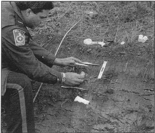
The sample can then be taken by slipping the sample container under the grooved out area and pushing up. The sample will fill the container with proper orientation. Excess material can then be struck off at the top of the container. In sandy soils, running the lip of the container upward along the face scrapes material into the container. By filling the container from the bottom of the horizon upward, the material orientation can be roughly maintained.
