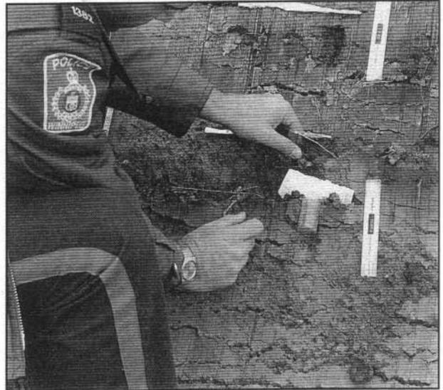
Samples can also be taken when lifting tape placed over the face. This method works especially well for sandy soils, less so for heavy clay. The tape should be placed over the horizon to be sampled and lightly pressed into the face. The tape can then be laid out on clear acetate in a similar fashion to lifting a latent fingerprint impression.
