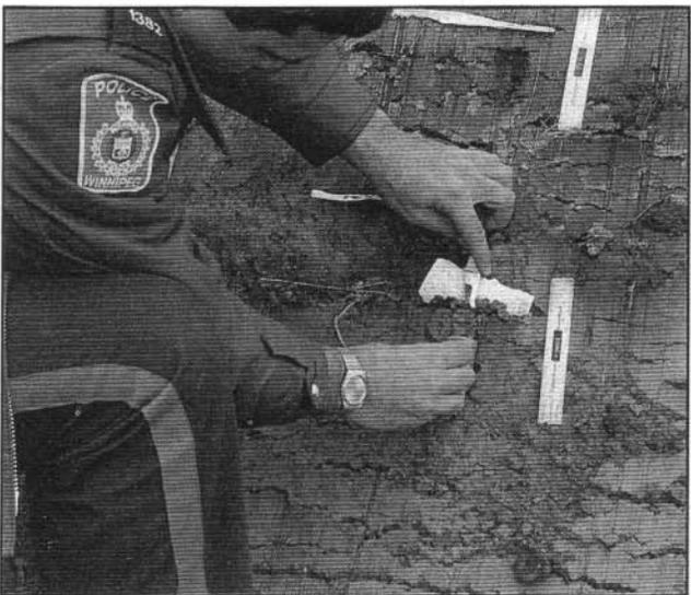
When a distinct boundary can be observed, a sample should be taken as closely as possible to the boundary. In hard soils, the sample can be cut out to fit the sample container and then allowed to fall into the container.
